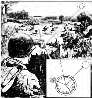
Figure 9. Sun and watch method of determining direction.
